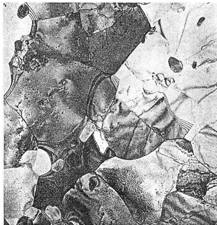
Fig. 3.6. Polycrystalline aluminium film, of almost uniform thickness. The different crystal grains appear light or dark depending on the crystal orientation with respect to the electron beam. Magnification 15,000 \times .
