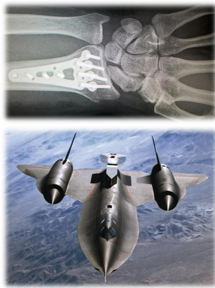
On most aircraft, use of titanium was limited by the costs involved; it was generally used only in components exposed to the highest temperatures, such as exhaust fairings and the leading edges of wings. On the SR-71, titanium was used for 85% of the structure, with much of the rest polymer composite materials.
