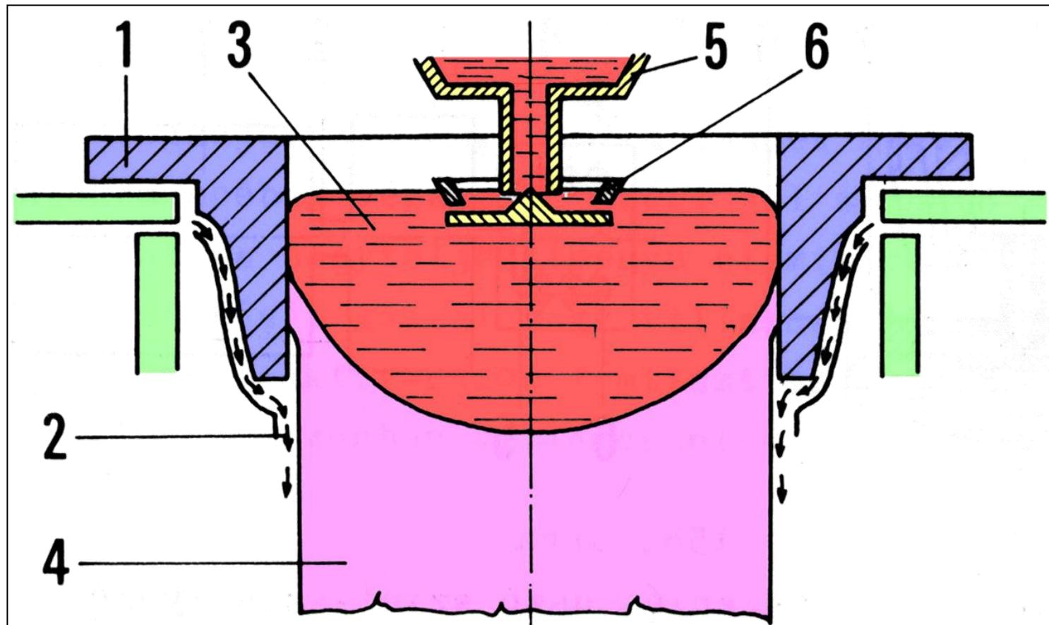
Pouring liquid metal continuously into a short mold (7.5–15 cm deep) that is open at the bottom. Only an outer layer of metal solidifies within the water-cooled mold. After leaving the closed mold at its bottom (e.g. with 5–15 cm/min), water is directly sprayed on the new ingot, continuing the solidification until complete (direct chill).
